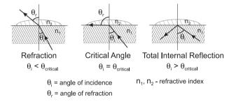
In the **HI 96802**, light from an LED passes through a prism in contact with the sample. An image sensor determines the critical angle at which the light is no longer refracted through the sample. The **HI 96802** automatically applies temperature compensation to the measurement and converts the refractive index of the sample to Fructose concentration in units of percent (by weight).
